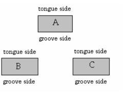
Two of the remaining boards (B & C) have their tongues removed and corresponding grooves inserted in the foam part of the LIGHT**GUARD** / HEAVY**GUARD** so that both the 4' long edges are grooved on both sides. This can easily be done with a handheld hot knife containing a long blade bent to conform to our factory groove. Boards "B" & "C" should have a cross-sectional profile as shown below.
