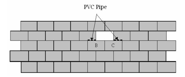
Finally, board "A" is installed into the hole with the tongue in its normal position. Using a knife blade, the PVC pipes are slid 12" laterally forming a partial tongue that will prevent the system from coming apart. This securement replacement is to be used for replacement boards in the field of the roof and is not intended as a possible replacement for normal securement as described in Technical Data Sheet 4.4.
