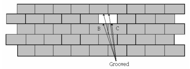
Two pieces of <sup>3</sup>⁄<sub>4</sub>" plumbing PVC pipe are cut 24" in length. These pieces of pipe are the replacements for the missing tongues in the system. The 24" pieces are slid in the holes formed by the removed tongue/fabricated groove openings of "B" & "C" above, as indicated by the illustration below.
