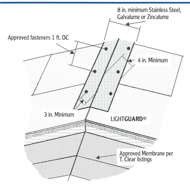
A minimum 8-in. wide metal strap, bent to conform to the angle change, is centered on the break line. The metal is secured to the LIGHTGUARD with approved fasteners spaced 1 ft. OC. The strap must extend a minimum of 4 in. onto the face of the LIGHTGUARD, with the fasteners secured a minimum of 3 in. from the edge of the LIGHTGUARD panel.
