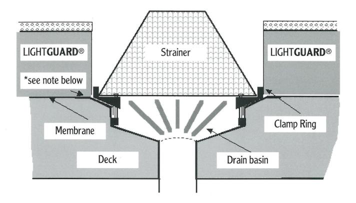
\*NOTE: This is not a flashing detail specification. Consult specifications for approved manufacturer's adhered or loose-laid membranes.
