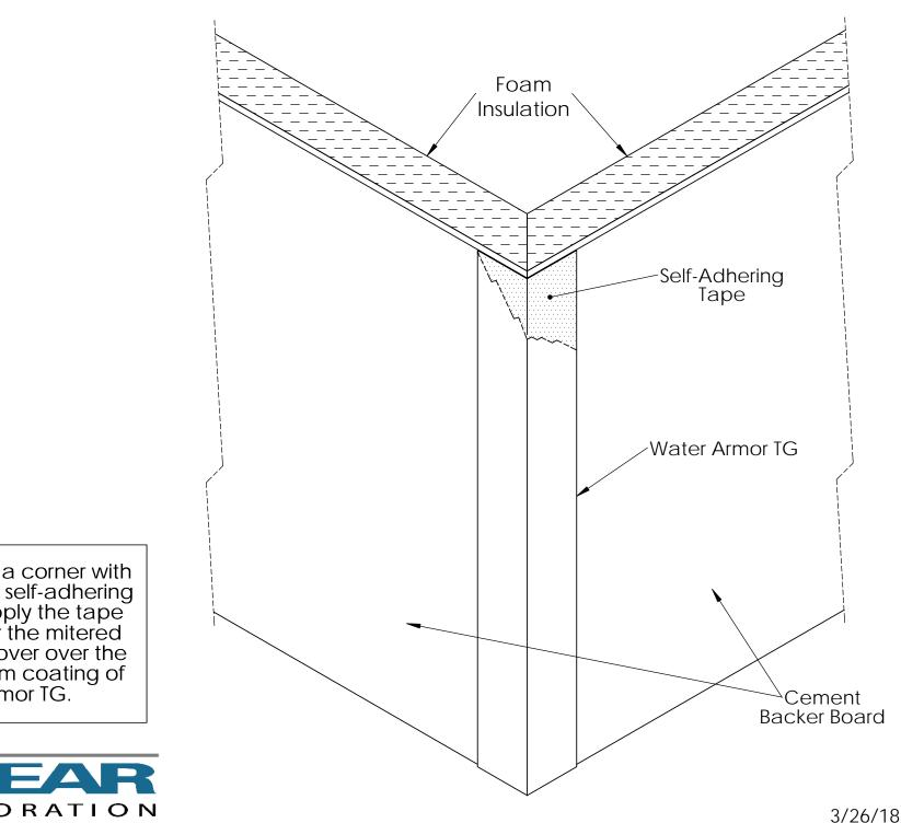
When creating a corner with ProGuard using self-adhering mesh tape, apply the tape centered over the mitered corner. Then cover over the tape with a skim coating of Water Armor TG.
