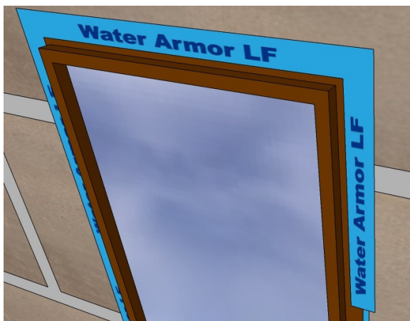
Window Flange Transition, strip in window following manufacturer's flashing recommendations.
