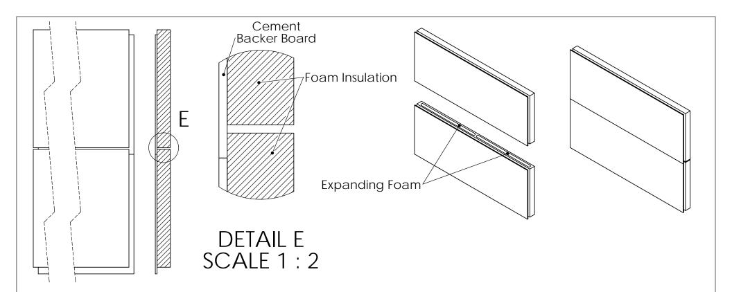
If the cement backer board meets flush with the connecting backing board and there is a gap between the foam, use expanding foam such as Fomo, or a similar polystyrene compatable expanding foam, to fill the area. Make sure to smooth the excess foam to be flsuh with the foam side.
